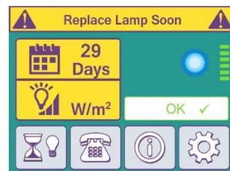
The user will be notified if a lamp failure occurs. Upon a lamp failure condition, the alarm relay will energize to close the outlet solenoid valve (optional) on the system and an audible alarm will sound. Replace lamp if needed
