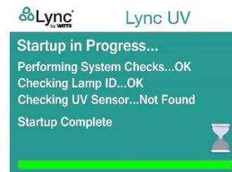
The lamp identifies it's self via radio frequency. If the wrong lamp is used in a system, this message will appear during start up.
