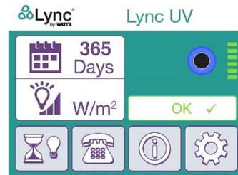
If the system detects low UV intensity, a yellow warning will appear. If the UV intensity is too low for safe operation a red warning will appear. In either condition the system should be checked immediately for proper operation.
