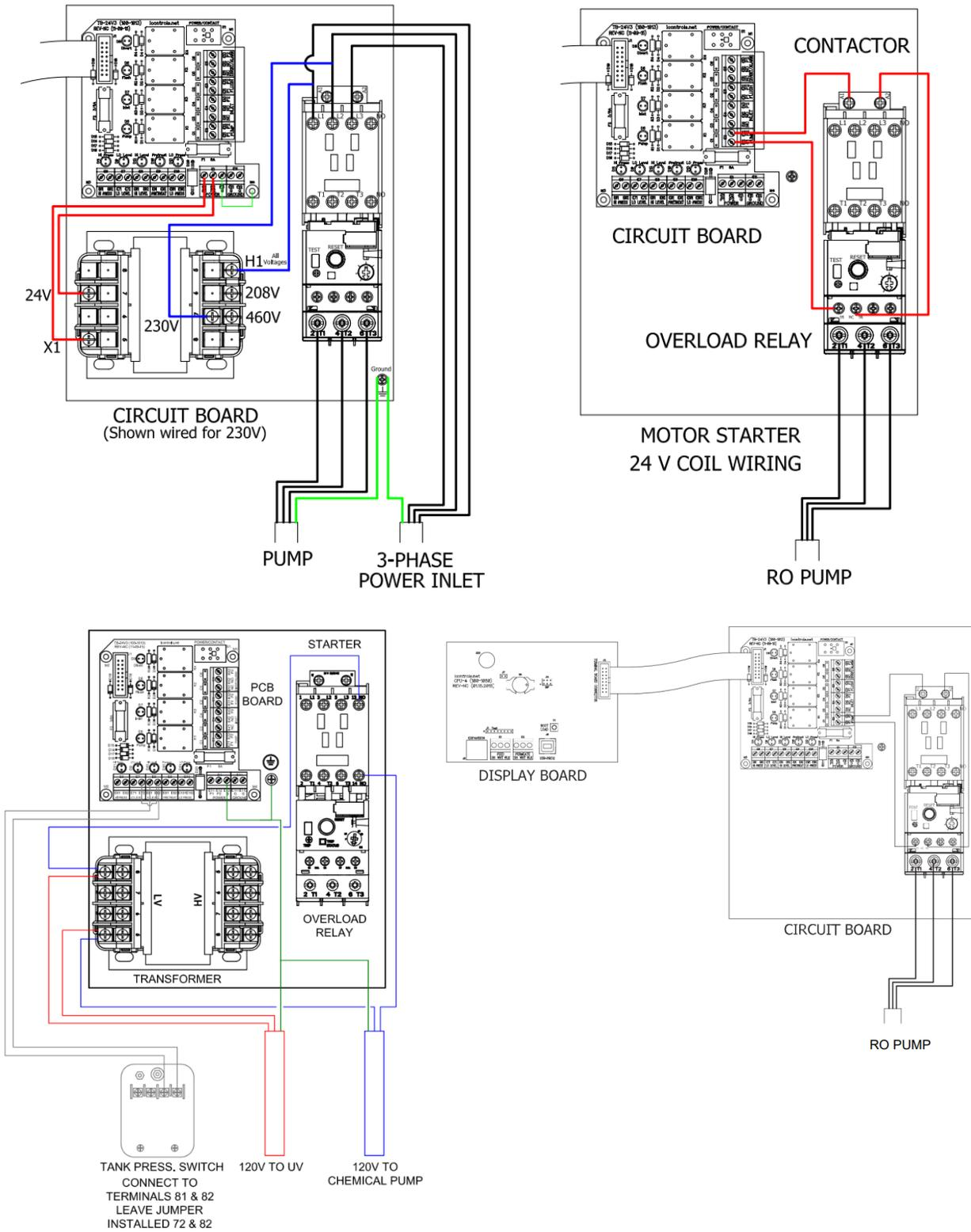
**Figure 2-4: Controller Wiring**
