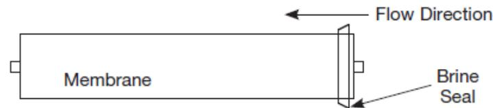
**Figure 6-1: Membrane Seal**
