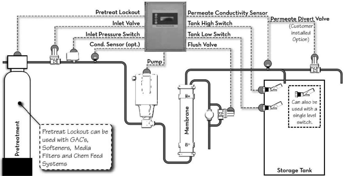
Figure 4-3: Wiring Diagram
