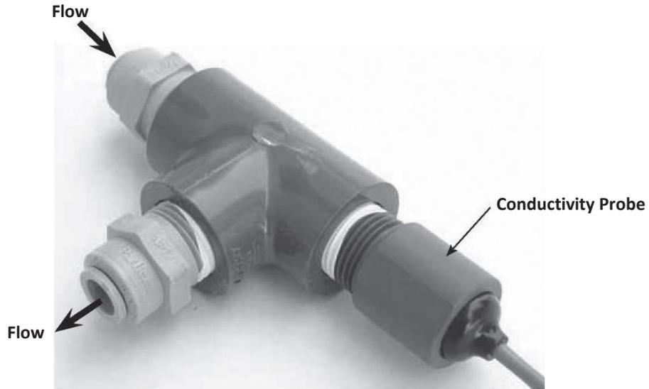
**Figure 4-6: Conductivity Probe Installation**
