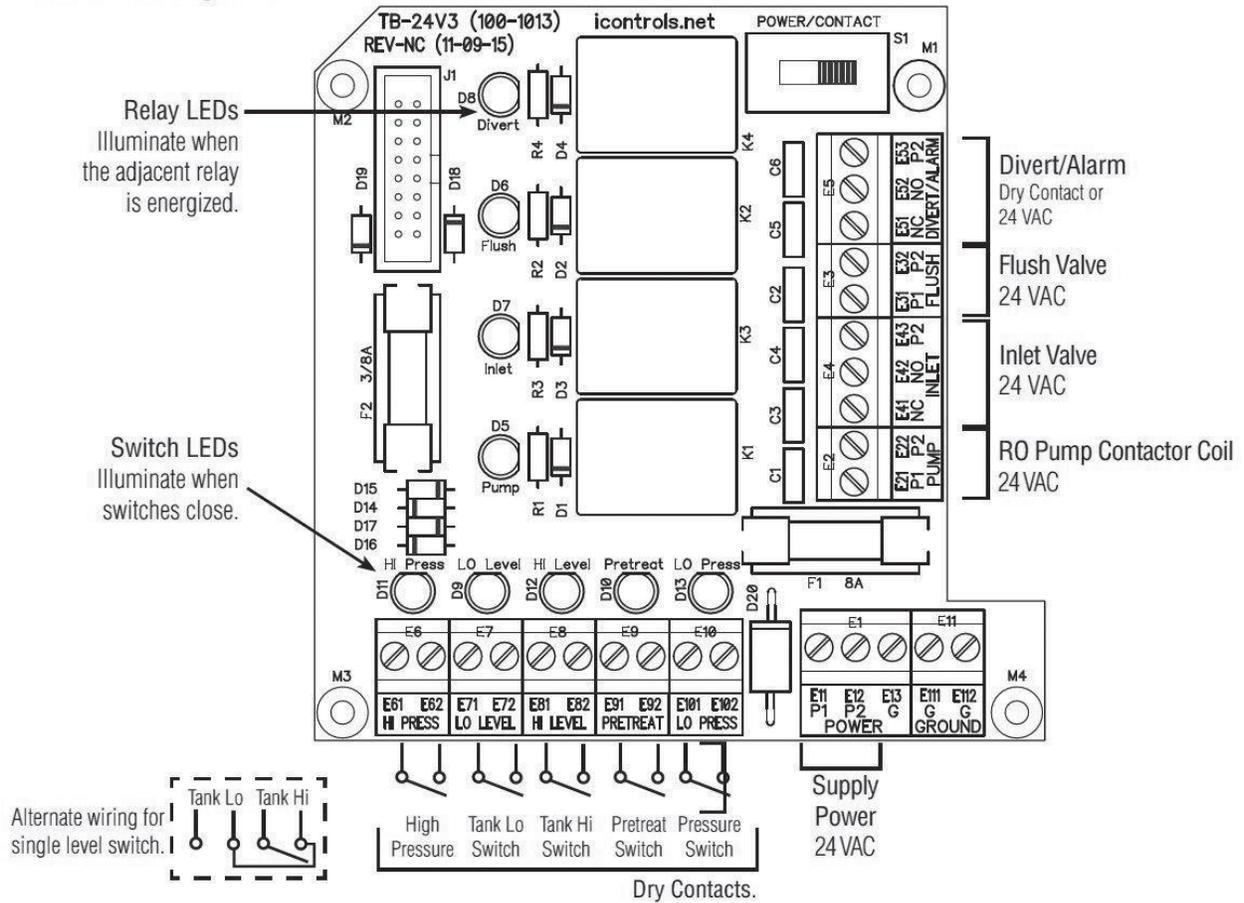
Figure 4-5: Controller Detail: Terminal Board, TB-3
