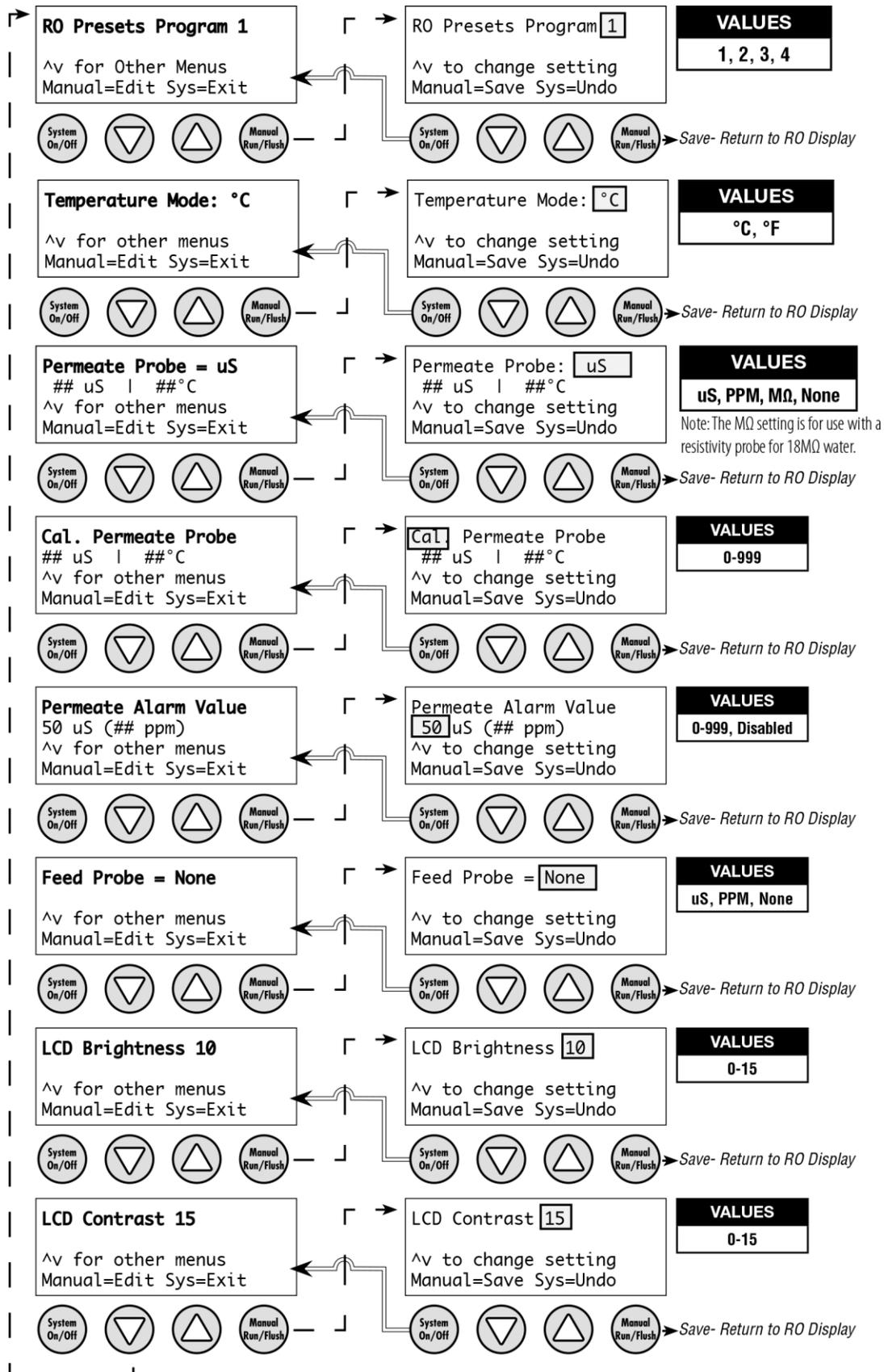
Figure 4-9: Controller Programming: Menu Navigation
