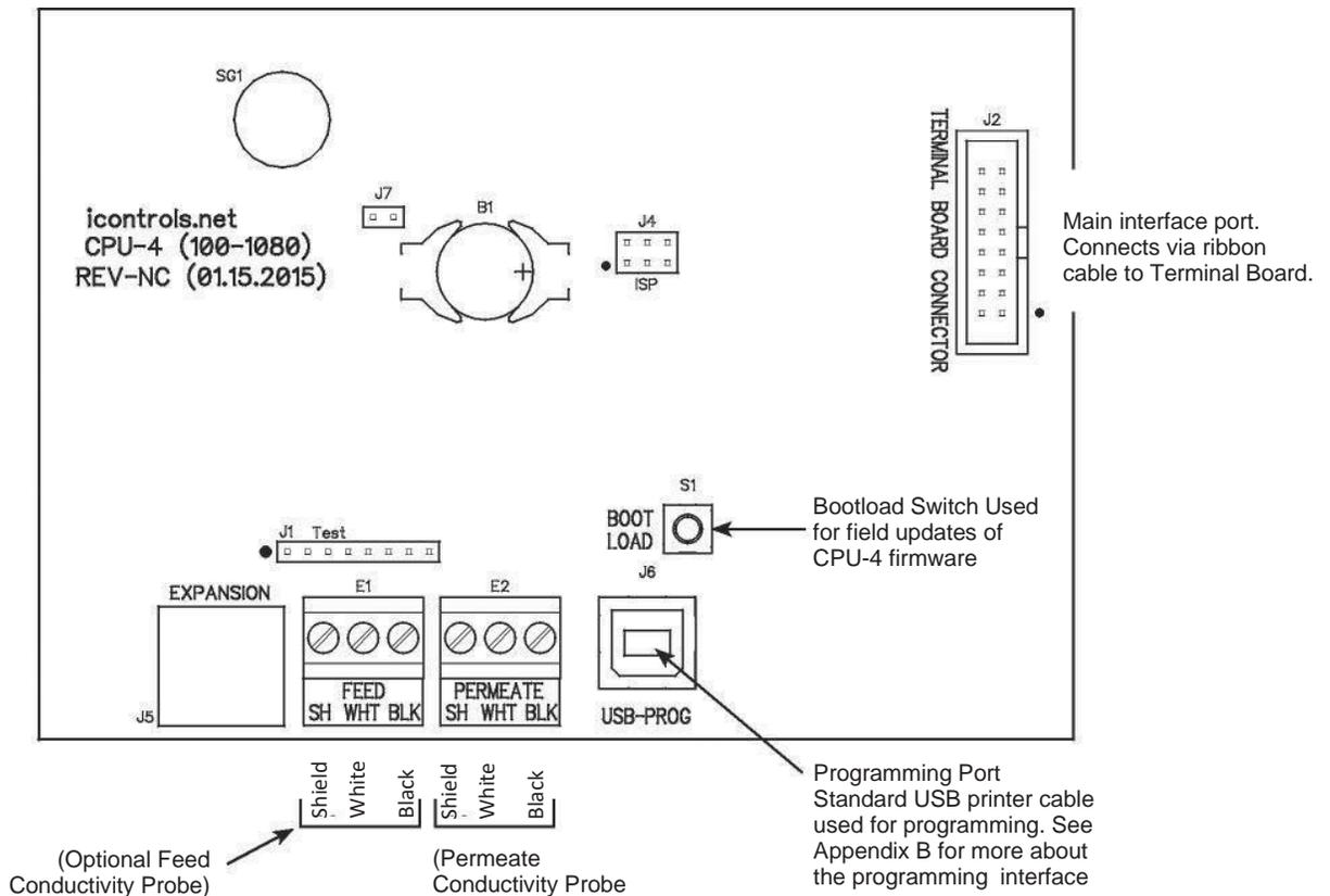
Figure 4-4: Controller Detail: CPU-4
