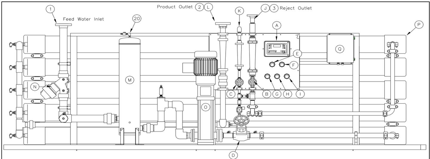
**Figure 2-3: WQRS-090-R, -180-R Systems Component Identification**
