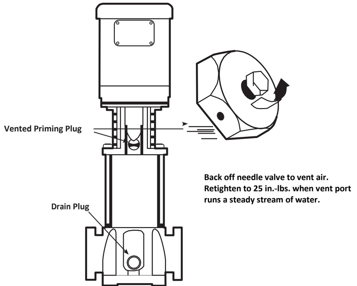
**Figure 3-1: Needle Valve Location**
