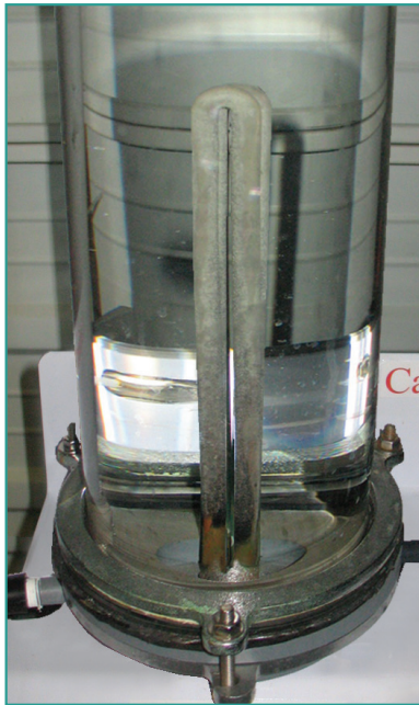
Untreated Scale build-up in untreated water
