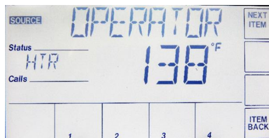
Figure 10-8 Setting the Setpoint
