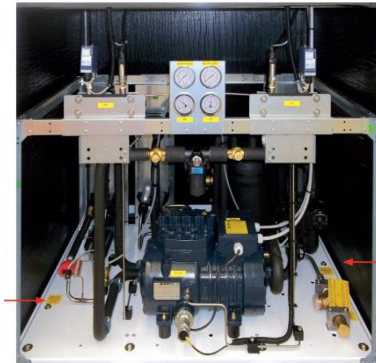
Figure 6: Transport Screw Locations
