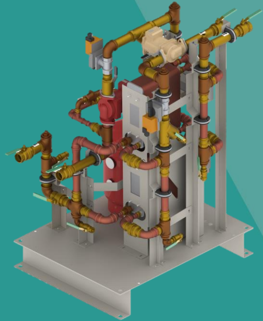
Dual Heat Exchanger
