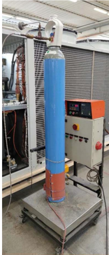
R-744 Cylinder with Heating Blanket and Scale
