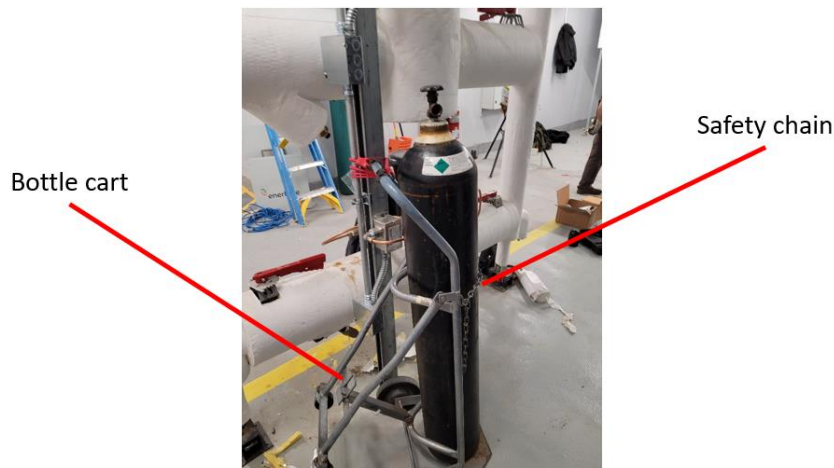
Ratchet straps or safety chains used to safely secure tank to cart
